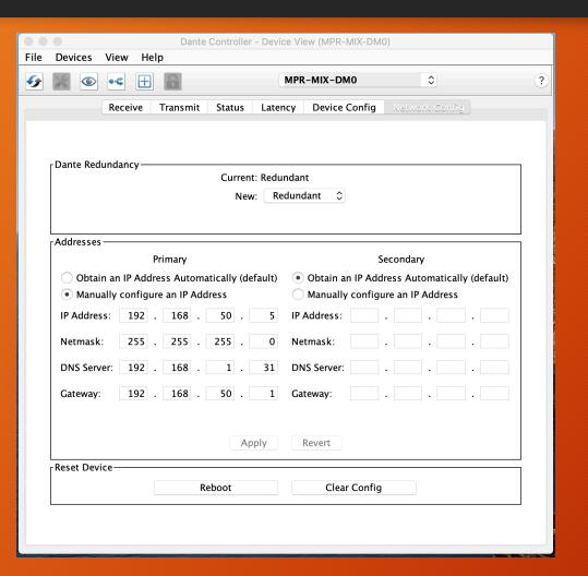
The Device View Network Config tab allows configuration of the dante redundancy (secondary) port as well as setting static IP address information or setting the ports to DHCP.
