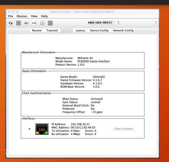
The Device View Status tab displays model and firmware information about your dante device as well as network interface information
