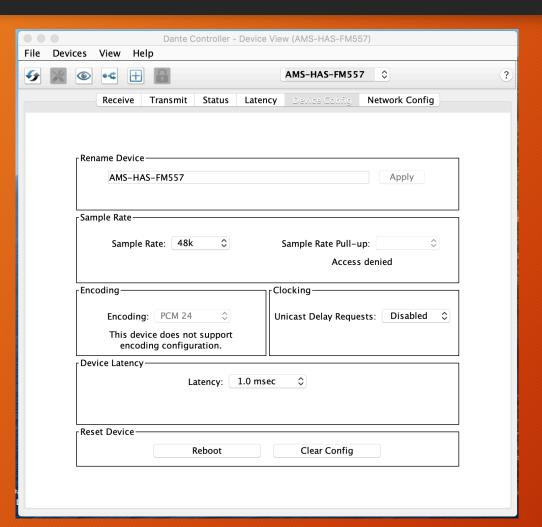
The Device View Device Config tab allows configuration changes to your dante device including renaming the device, changing the sample rate, PCM encoding, latency as well as the ability to reboot the device
