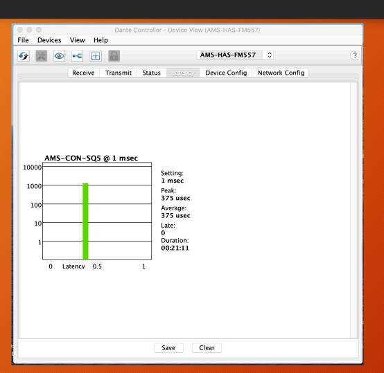
The Device View Latency tab displays current latency settings as well as network utilization information
