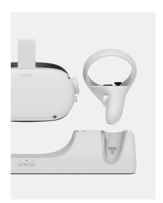
2. Headset must *click* to the charging adapter. If these two pieces are not together, the headsets *will not charge*.
